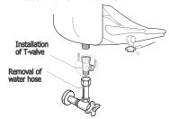
Remove the existing water hose and then install T-valve to the bottom of the toilet tank. Ensure the rubber washer is properly seated and attach the original water hose to the T-Valve.
