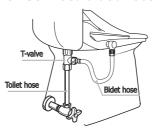
After installing the T-valve, connect the supplied bidet hose from the center of the T-valve to the bidet.
